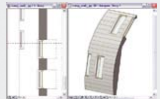
Correct openings representation in all wall shapes
